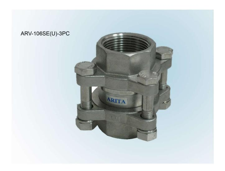
The design of Arita 3 Piece Disco Check Valves is compact and is meant for screwed ends connection. The parts are produced using investment casting which contributes to its high quality finishing and precision. The design allows it to be installed either in horizontal or vertical position. The 3 Piece Disco Check Valves have a wide range of applications like with steam, hot condensate, water, oil and gas.
