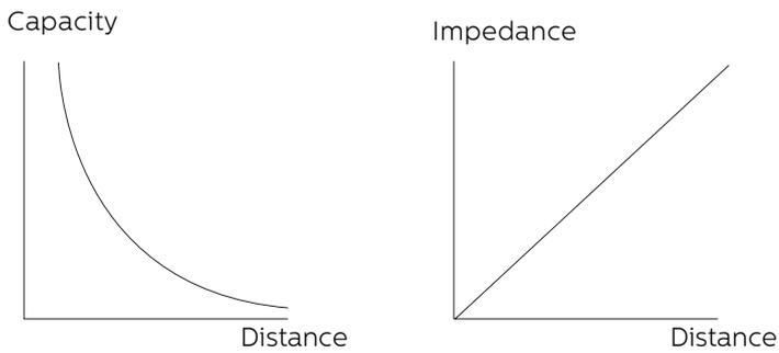
Impedance is  $Z = R + jL\omega + (jC\omega)^{-1}$ . R is defined as reel component and represents the medium conductivity.
