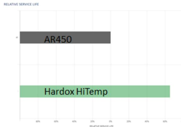
Hardox® HiTemp performs 60% better than AR450 when the temperature is 500 °C
