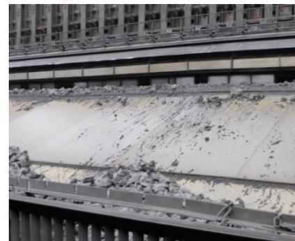
Liner plates in coke plant cooling bed
